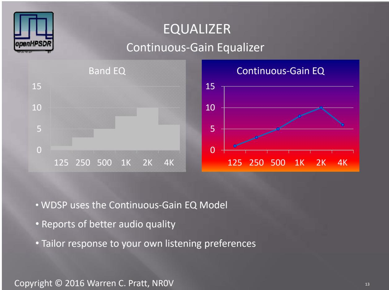
The slide features the 'openHPSDR' logo in the top left. The main title is 'EQUALIZER' with the subtitle 'Continuous-Gain Equalizer'. Two graphs are shown: 'Band EQ' on the left and 'Continuous-Gain EQ' on the right. Both graphs plot gain (0 to 15) against frequency (125, 250, 500, 1K, 2K, 4K). The Band EQ graph shows a step-like response, while the Continuous-Gain EQ graph shows a smooth curve. Below the graphs is a bulleted list of features.
