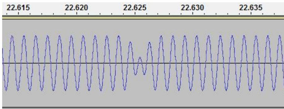
Since these actions involve half the samples in the ring buffer, they are substantial and the sound of the disturbance is not totally masked. However, in all cases, discontinuities in the sample stream have been avoided and the high-frequency "pop" energy caused by such discontinuities is eliminated.
