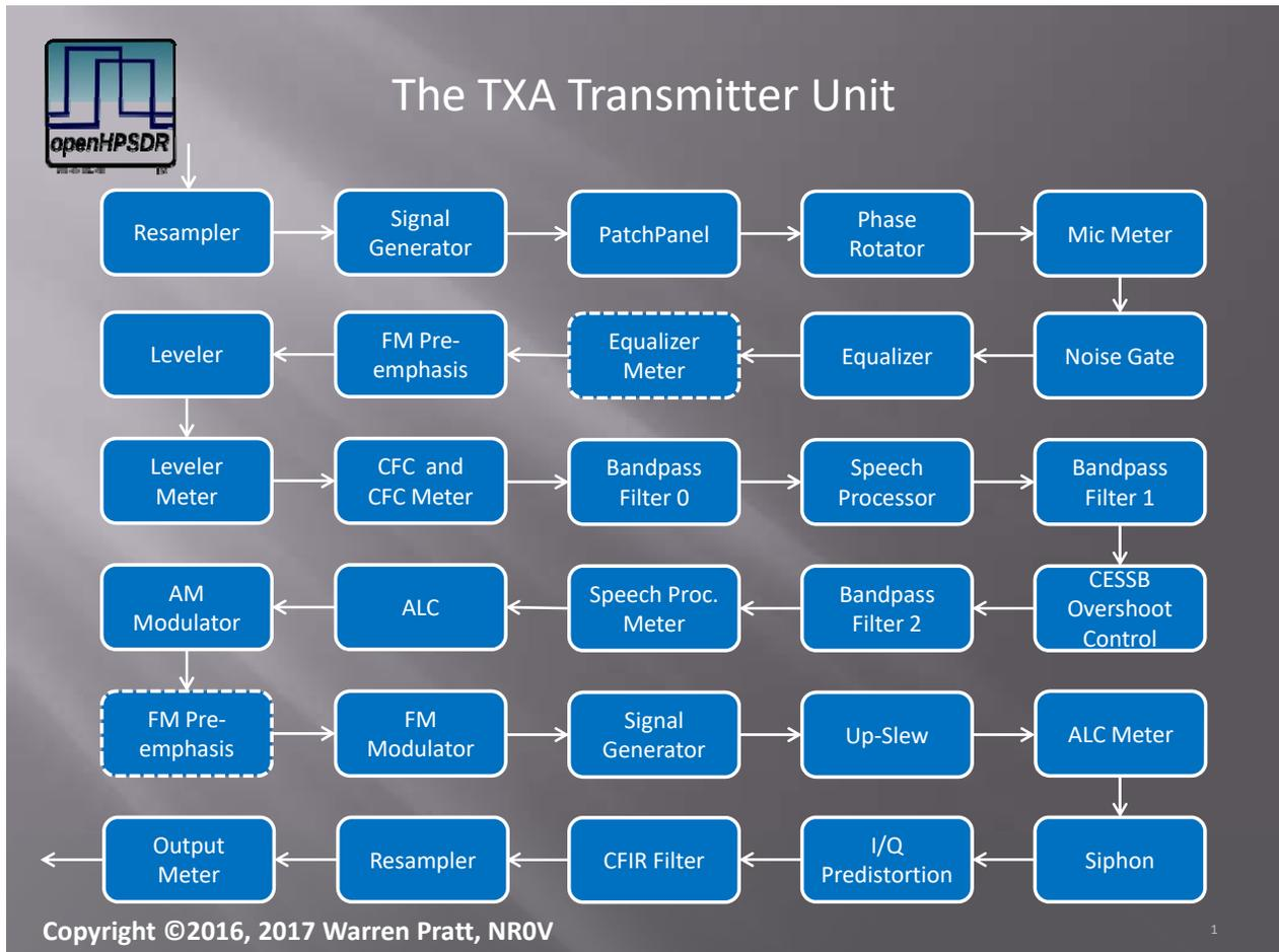
The above figure displays the arrangement of blocks in the TXA transmitter unit. We will now discuss the operation and control of each block.
