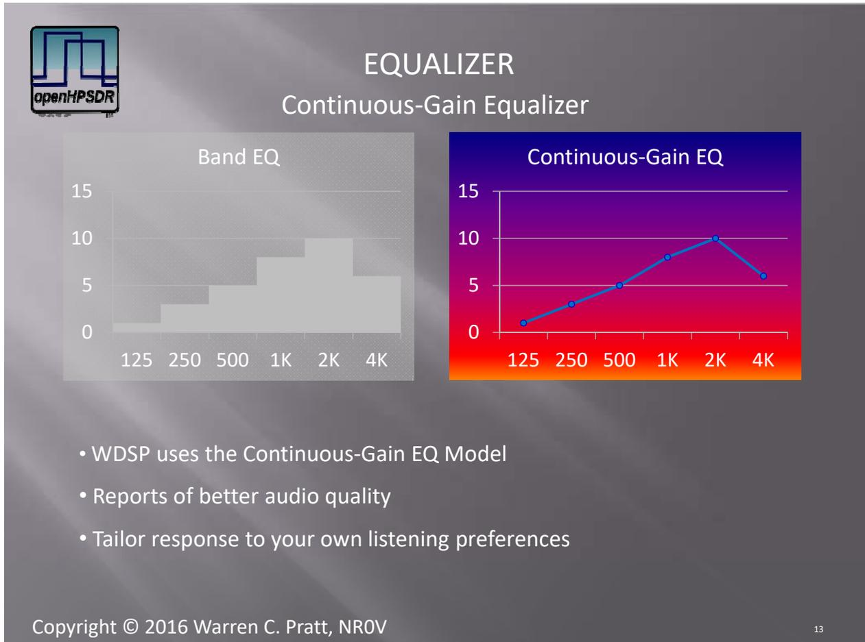
The slide features the 'openHPSDR' logo in the top left. The main title is 'EQUALIZER' with the subtitle 'Continuous-Gain Equalizer'. Two graphs are shown: 'Band EQ' on the left and 'Continuous-Gain EQ' on the right. Both graphs plot gain (0 to 15) against frequency (125, 250, 500, 1K, 2K, 4K). The Band EQ graph shows a step-like response, while the Continuous-Gain EQ graph shows a smooth curve. A bulleted list and copyright information are at the bottom.
