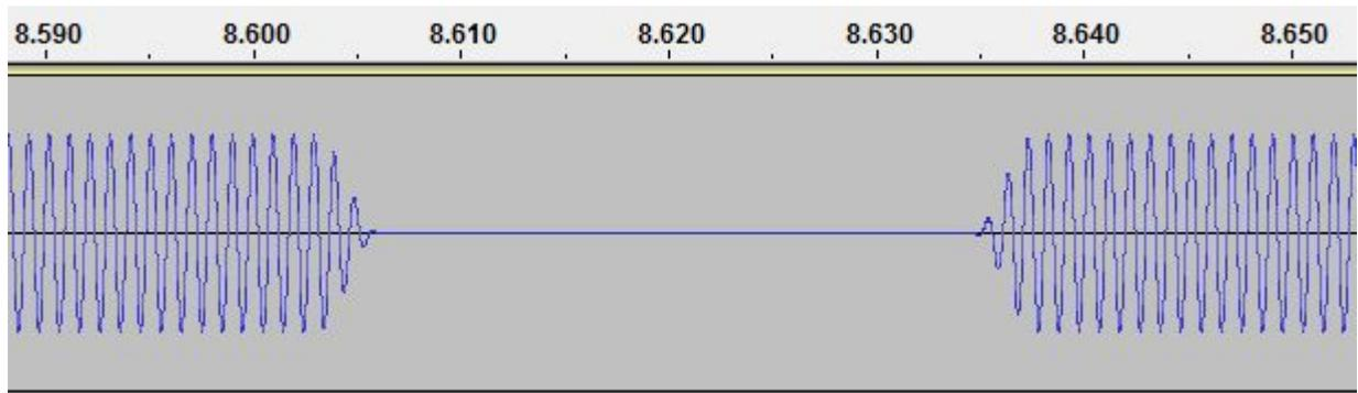
In an overflow situation, half of the samples in the internal ring are discarded so that another overflow will not occur if the next write occurs before a sufficient number of samples are read. In that case, the waveform before the discarded samples is "blended" with the waveform after the discarded samples.
