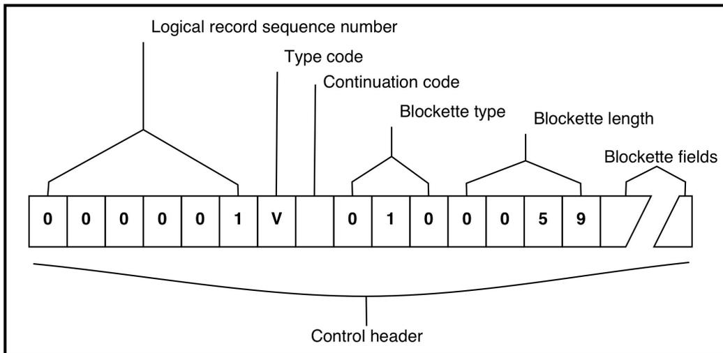
Figure 10: Beginning Fields of a Control Header
