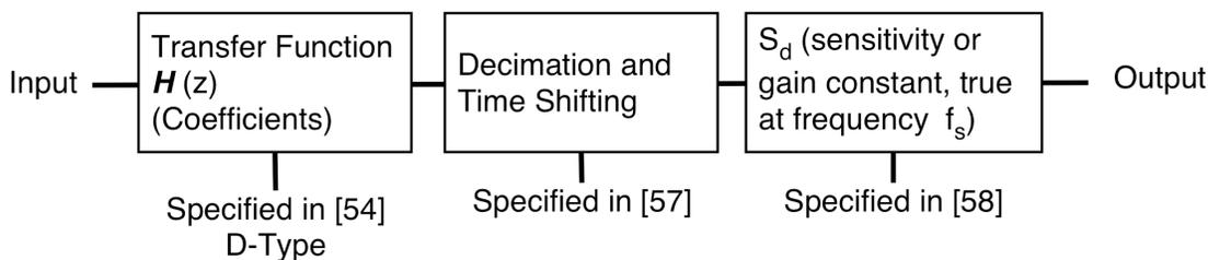
**Figure 8: Example Digital Stage Using Coefficients Representation**
