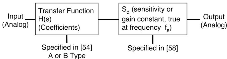
**Figure 7: Example Analog Stage Using Coefficients Representation**
